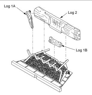
Figure 29 - Installing Logs 1A, 1B and 2
